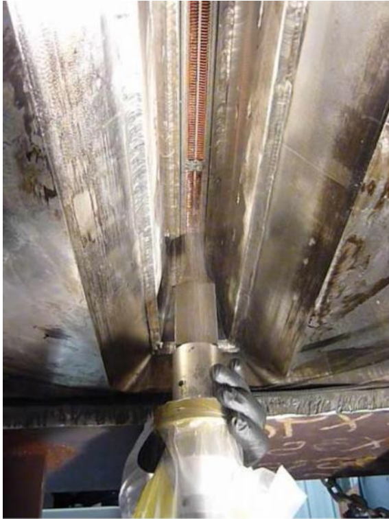
Ultrasound (22 kHz, 1000 W) applied to outlet face results in discharge
